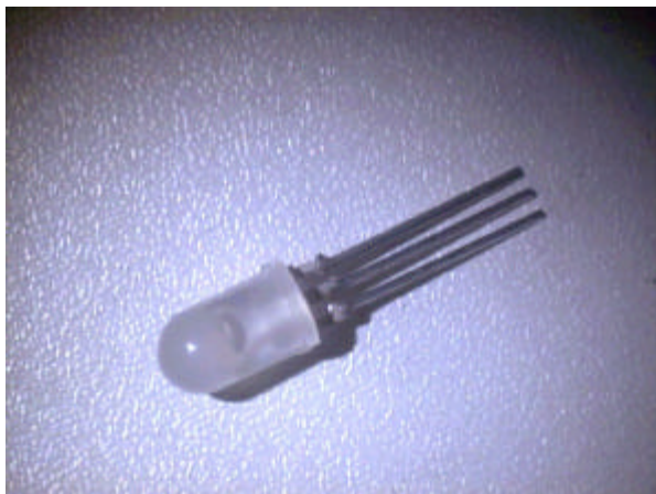
Fig. 1 a two-color LED
