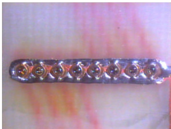
Pic 7 A homemade phototransistor line in 1/10" raster for 8 bit
