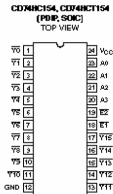
Pic 2 Connection diagram of 74HCT154
