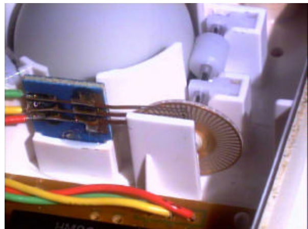
Fig. 2 Scanning with segmented disc
