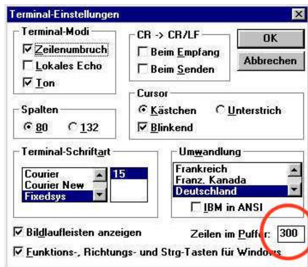
Fig. 9 Set buffer to 300 lines
