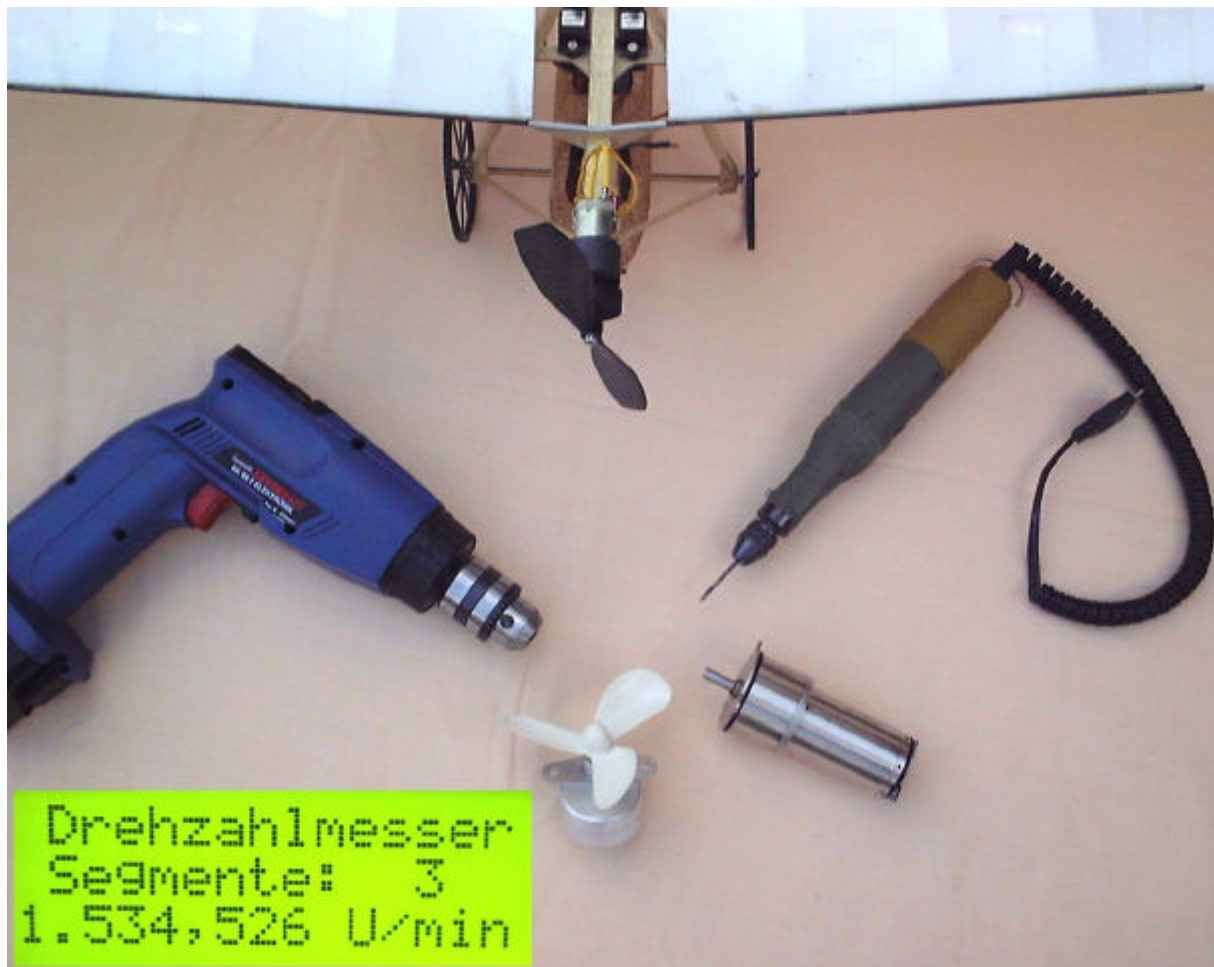
Fig. 1 The BASIC-Tiger® measures the revs per minute of several items using little hardware and software.
