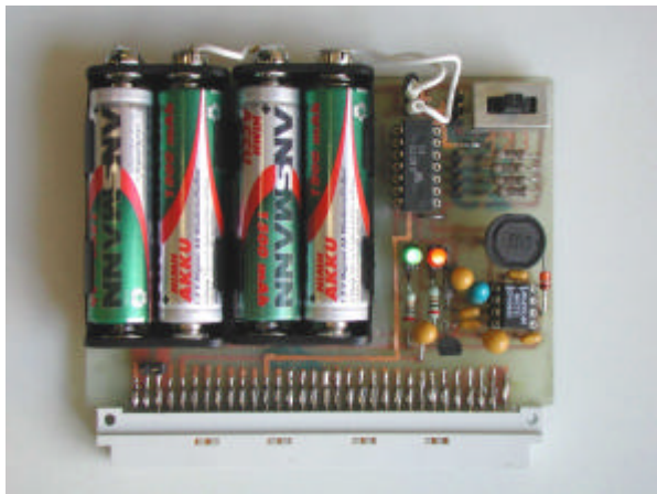
Fig. 6 Battery module with sleep and wake circuit
