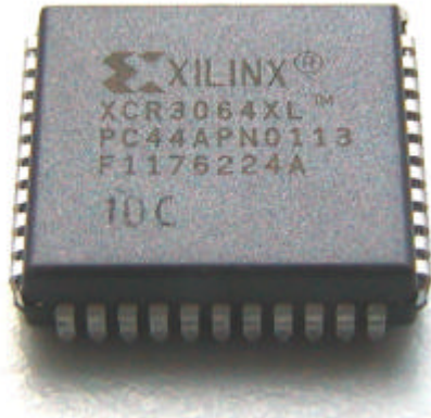
Fig. 2 The XCR3064XL in a 44 pin PLCC package Fig. 3 A self-made programming adapter package
