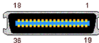
Fig. 2 Centronics plug (Type B, printer side)
