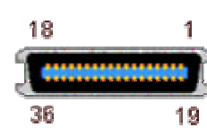
Fig. 3 Miniature Centronics plug (Type C, printer side)
