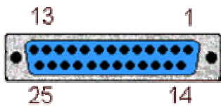
Fig. 1 25-pin SUB-D socket (Type A, PC side)
