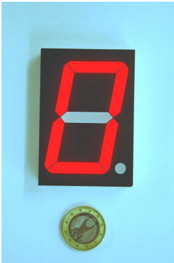
Fig. 1 A 7-segment large display in comparison with a EURO coin
