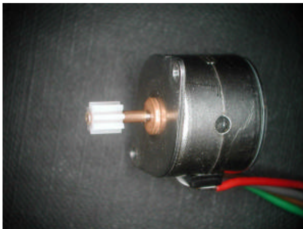
Fig. 3 You can fit the pinion to the motor shaft using a small metal capsule or a heat-shrinkable sleeve
