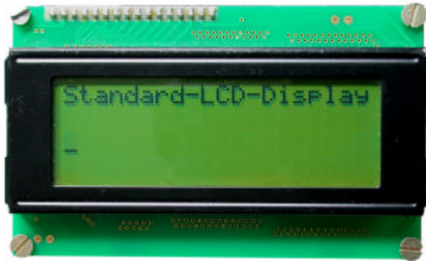
Fig. 1 the familiar 4-lined Plug-and-Play-Lab LC display
